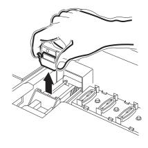
4. Hold the projections at both end to insert a new wiper.
