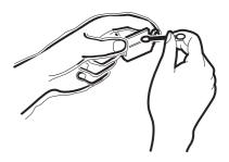
9. Holding the projections at both ends, insert the wiper which has cleaned into place.
