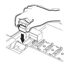
11. Wipe off ink or dirt adhered to the rubber of the cap and the ceiling of the wiper cover using cotton buds.
