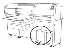
9. Unlock catch clips on both sides of the cover.
