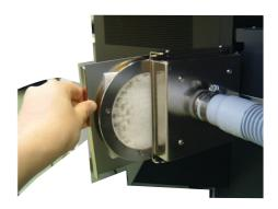
From the filter holder, remove the filter and replace with a new filter.
