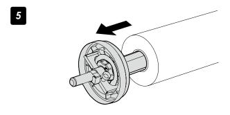
Supporting the scroller flange, pull out the scroller shaft.
