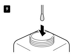
Dip a cleaning swab in the cap cleaning liquid.
