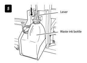
Lower the lever, and make sure that the splash guard was lowered.
