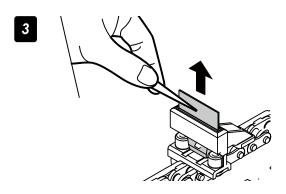
Then pull the wiper blade out from its slot.
