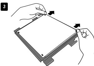
Remove all wrinkles on the head cleaning sheet by lightly pulling both sides of the sheet top edge in the direction of the arrows. This will prevent the sheet from rising near the bottom edge attachment locations.
