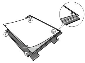
Place the head cleaning sheet on top of the support sheet. Hook two holes to the attachment locations (a) and (b) and then the two others holes to the attachment locations (c) and (d).
