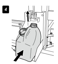
Slide the lever up and install a empty waste ink bottle.
