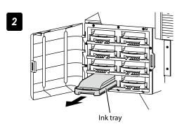
Confirm the color of the ink pack to be replaced, and pull its ink tray out of the Printer.
