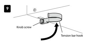
Loosen the knob screw of each tension bar hook and extend it laterally.
