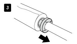
Remove the flange spacer.
