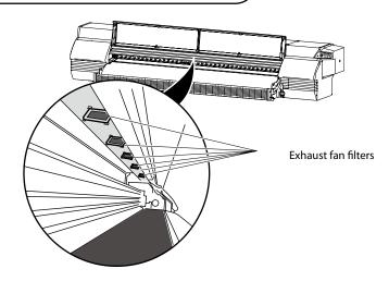
When replacing the exhaust fan filters from the operation panel menu, start the procedure from step 1. When replacing while executing **[#START MAINTENANCE]**, start the procedure in step 6.
