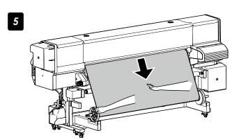
Rotate the scroller flange manually to take up the media.
