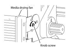
(2) Loosen the right and left knob screws next to the movable media drying fan.
