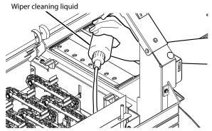
When the cleaning liquid level is lower than the "X" mark's top edge, replenish the wiper cleaning liquid.
