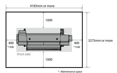
Secure 2200 mm in horizontal direction. (Unit: mm)
