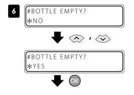
On the operation panel, select "YES" and press the key to reset the waste ink counter.
