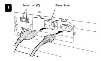
With the two power cords supplied with the Printer, connect the Printer's two power inlets and the power supply's two sockets.
