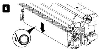
By pressing the key feed the media, and wind one full turn of the media on the paper tube.
