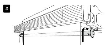
Place the take-up side tension bar at the tension bar hook.
