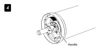
At the other side, rotate and loosen the scroller flange's handle.
