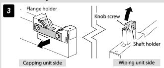
Remove the flange holder, and open the shaft holder.
