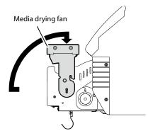
(3) Pull the media dryer fan toward you, and turn it upward by 90 degrees.
