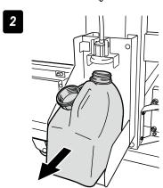
Carefully pull out the full waste ink bottle, taking care not to spill any on the printer or on the floor.
