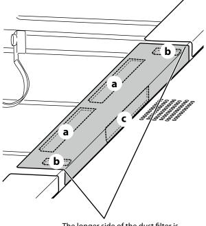
The longer side of the dust filter is slightly longer than the sheet metal.
