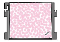
Apply 4 cc of wiper cleaning liquid on the head cleaning sheet surface using a dropper. Apply 1 cc four times as follows.
