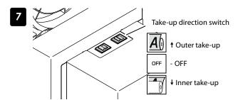
Set the take-up direction switch according to the take-up direction.
