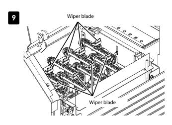
Visually check the wiper blade for contamination and scratches.
