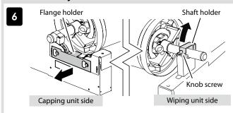
Remove the flange holder, and open the shaft holder.
