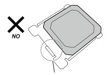
The filter does not touch the shorter filter guide.
