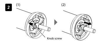
Remove the scroller shaft fixture at one side.
