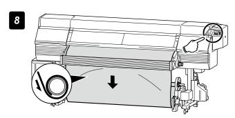
By pressing the key feed the media, and wind one full turn of the media on the paper tube.
