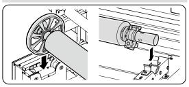
Load the media roll into the Printer's rear side (supply side).
