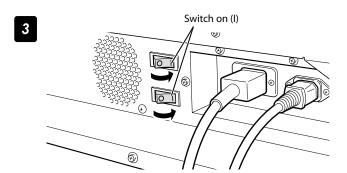
Set the printer power switch and heater power switch to on, the side marked with I.
