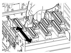
Clean the top surface of the cap by rolling the cleaning roller.
