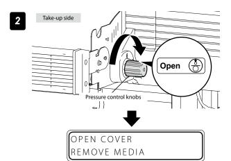
Rotate the pressure control knob, and set it to "Open", and then open the front cover.
