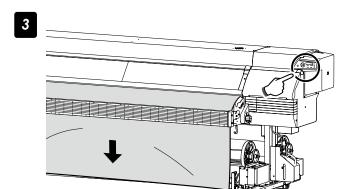
By pressing the key, feed the media until the front media edge is wound on the paper tube.
