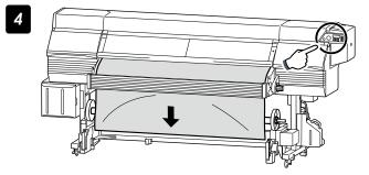
By pressing the \(\sigma\) key, feed the media until the front media edge is wound on the paper tube.
