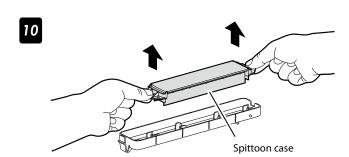
Set a new spittoon case's locating hole to the protrusion, and fix it horizontally by pressing slightly.
