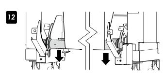
Place the tension bar at the bottom of the tension bar guide.
