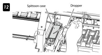
Confirm that the spittoon absorber liquid's top surface is as high as the top of the protrusions.
