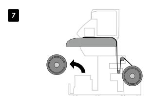
When the media is installed on the take-up reel unit, remove the media.
