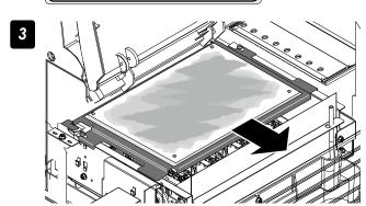
Remove the sheet cleaning part on the top of the wiping unit, and then close the covers.
