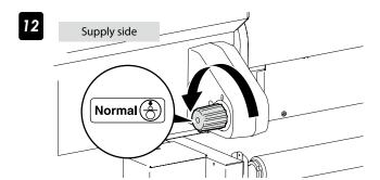
Set the pressure to "Normal" by rotating the pressure control knob counterclockwise.
