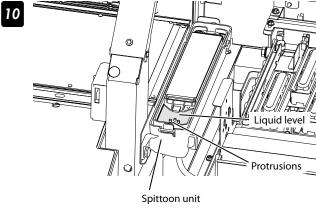
Pour the spittoon absorber liquid into the spittoon case until the liquid level is as high as the indication protrusions.
