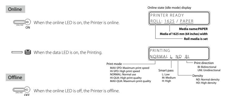
The Printer in offline displays the menu group on the LCD, and activates the menu operation.
