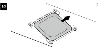
Remove the old exhaust fan filters.
