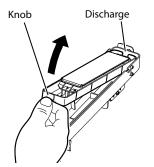
Press the knob at the near side of the case containing the spittoon absorber liquid to open the lid, raise the front side of the spittoon absorber liquid case to discharge the spittoon absorber liquid to the backside.
