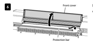
Remove the protection bar and open the front cover.
