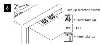
Set the take-up direction switch according to the take-up direction.
