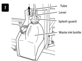
Slide the lever up and lift the splash guard sufficiently to remove the waste ink bottle.
