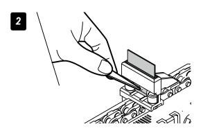
Using the tweezers, remove the wiper blade. First pull the bottom of the wiper blade to release the hook of the plastic projection.
