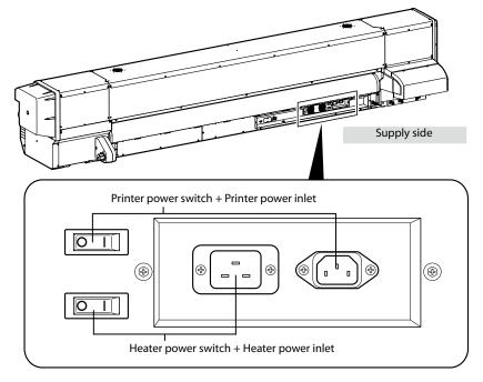
Turn the printer power and heater power switches on only before your first operation. From the next operation, turn the Printer on and off only by pressing the POWER switch on the operation panel.
