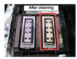
Important! At this point, clean the cap rubber only. Do not clean the mesh inside the cap. Execute "DISWAY WASH" regularly (about once a week) to clean the mesh inside the cap. (Refer to "Operation Manual" chapter4)
