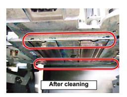
**Capping station ("Cleaning the Wiper and Cap" Chapter 4 of the Operation Manual)** The surrounding area of the cap is also liable to be stained by the dust and ink. It is recommended to clean the head frequently using the cleaning liquid for maintenance suitable for the ink used to avoid the stains on the head.
