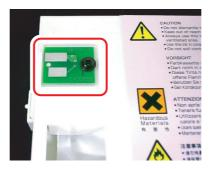
The board mounted on the ink cartridge
