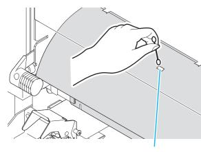
Cleaning of the media sensor at the rear surface of the machine
