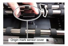
2 Loosen the screws retaining the origin mark sensor.
