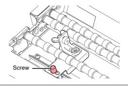
**2** Lightly loosen the screws (2 pieces) retaining the right work holder.
