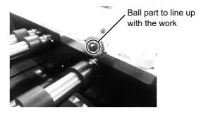
Tighten the screws (2 pieces) retaining the right work holder.
