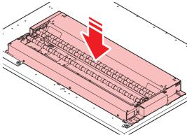
(4) Fix the Kebab MkII L system into place with a plastic knob screw while pressing it into the K positioner BKT\_R side.
