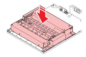
(5) Fix the Kebab MkII system into place with a plastic knob screw while pressing it into the K positioner BKT\_R (L) side.
