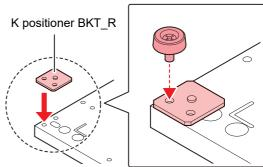
(3) Attach the cable BKT in the back of table.
