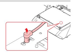
4 Remove the table by lifting up.
