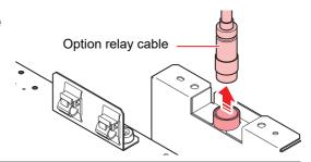
**5** Remove the option relay cable from the rear surface of Kebab MkII system.
