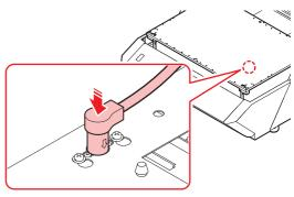
**14** Remove the K positioner BKT\_R (x2) at the both front edges of table.
