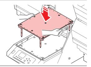
**12** Remove the K positioner BKT\_R (x2) at the both front edges of table.
