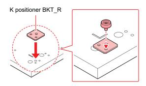
(2) Attach the K positioner BKT\_for 7151 in the left front corner of the table using a provided plastic knob screw.
