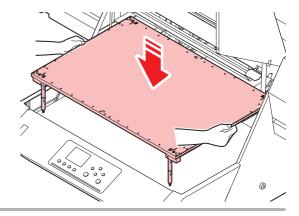
13 Put the cable under the table into the printer main unit.
