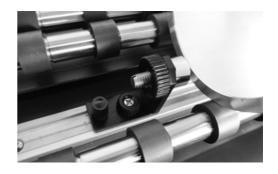
10 Tighten the screw of the left work holder.
