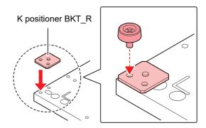
(3) Attach the cable BKT in the back of table.
