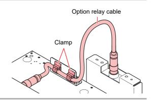
Remove the option relay cable from the printer main unit.
