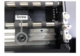
Align the positions of the origin mark of the work and the origin mark sensor.
