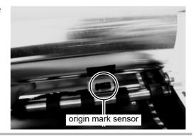
5 Tighten the screws and fix the origin mark sensor.
