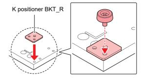
(2) Attach the K positioner BKT\_R in the left front corner of the table using a provided plastic knob screw.
