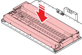
(5) Fix the Kebab MkII L system into place with a plastic knob screw while pressing it into the K positioner BKT\_R (L) side.
