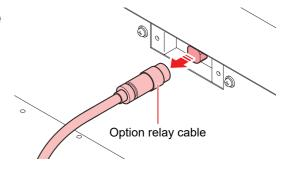
Remove the option relay cable from the rear surface of Kebab MkII system.
