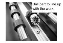
9 Slide the left work holder, and put the ball part of the left work holder lightly to the work.
