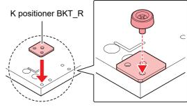
(2) Attach the K positioner BKT\_R in the left front corner of the table using a provided plastic knob screw.
