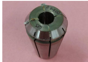
Debris accumulated in the chuck grooves
