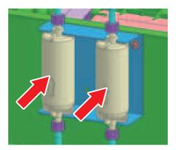
1 Tighten the fittings above and below the filter, and recheck to confirm that they are not loose.
