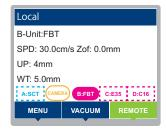
Press 🌢 👽 to select [Setup] > [Draw] > [Vacuum Auto-Off], then press the [ENTER] key.
