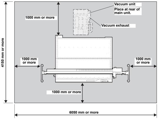
Note: Figure shows installation in the case of CFX-2513
