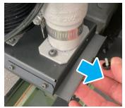
With an R10 fitted with a knob screw, removing the screw makes it easier to check and clean inside the dust collector box.
