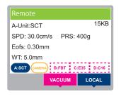
SPD: Cutting speed PRS: Cutting pressure Eofs: Offset value WT: Work thickness
