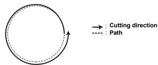
Values of circle θ correction are automatically calculated based on the radius of circles to draw.
