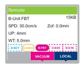
SPD: Cutting speed Zof: Z origin offset value UP: Up height WT: Work thickness
