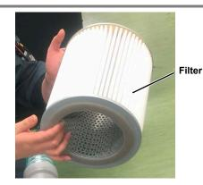
Vacuum the filter to remove dust or debris.
