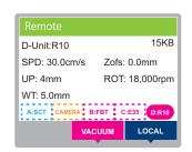
SPD: Cutting speed Zof: Z origin offset value UP: Up height ROT: Rpm WT: Work thickness
