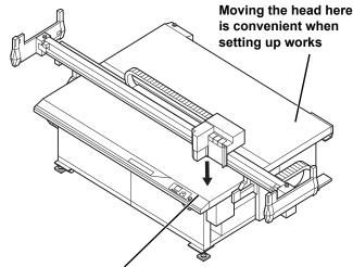
Moving the head here is convenient when mounting tools
